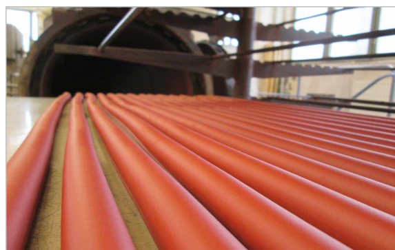
Preparation for vulcanization
